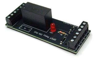
A single DPDT ready assembled relay module mounted on a small PCB. All connections are made via screw terminals and it has LED indication to show when the relay is activated.
