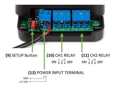
If the power supply is successfully connected, the power LED (5) will light up and the TUYA LED (6) will start flashing after a few seconds.
