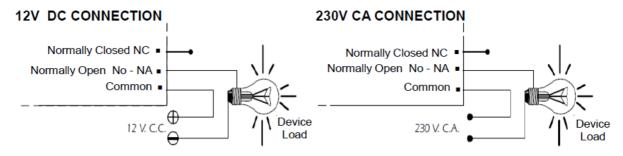
**INFORMATION ABOUT THE OUTPUT.** During the operating mode and according to its load, it could happen a fluctuation or an incorrect working of the output. In such case, you have to install an anti-spark circuit between both contacts of the used relay, as it is indicated on the schedule
