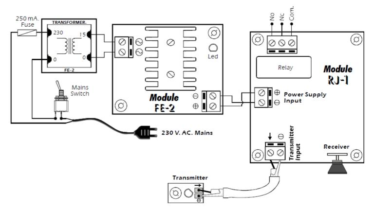
**OUTPUT CONNECTION.** The RJ-1 output is controlled by a relay, and accept any device up to 5 A. The relay have three output terminals: The normally open quiescent (NO), the normally closed quiescent (NC) and the common. This Mechanism operate like a switch with two terminals NC and Common. For the inverse function you have to use the NO and Common. In the drawing hereafter, you could see a typical connection with a 12 V D.C and 230 V A.C devices.
