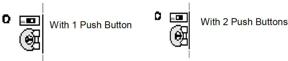
**OPERATION WITH TWO BUTTONS :** If you placed the microswitch on the OFF position, the On button connected to the input, while hold progressively increase the output signal. Pushbutton input connected to Off, however, remains depressed while gradually decrease the output signal.
