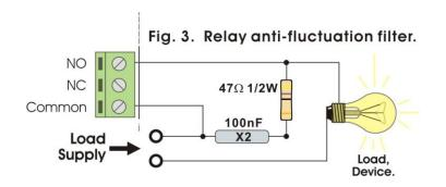
**<u>Note</u>**: To connect load at 12V DC, you have to remove the resistor and to only use the capacitor.
