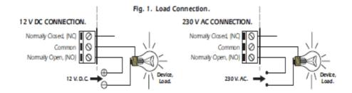
**INFORMATION ABOUT THE OUTPUT**. During the operating mode and according to its load, it could happen a fluctuation or an incorrect working o fthe output. In such case, you have to install an anti-spark circui tbetween both contacts of the used relay. If the load connected to the relay is supplied by 230V, you have to use a 100nF/400V Capacitor and a 47W. ½ W resistor, as it is indicated on the drawing herewith.
