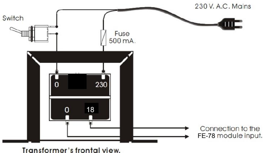
**MODULE CONNECTION:** Once you have completed the wiring of the circuit transformer '.
