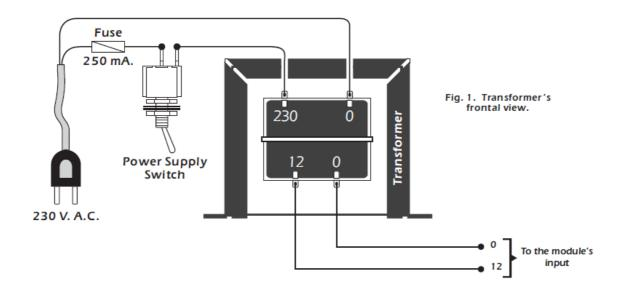
**MODULE WIRING.** Once the transformer's wiring done, you have to wire the module. Firstly, you have to check that there is no voltage (230 V AC) in the module.
