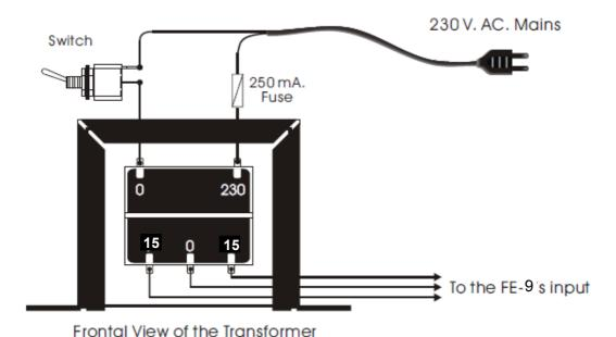
**MODULE'S CONNECTION.** Once the transformer's connection done, you have to verify that the module is not supplied by 230 V A.C. Connect three inferior terminals to the input module's terminals (15, 0 & 15) as it is indicated in the General Wiring Map. Activate the switch and Leds will light indicating that the module is operating.
